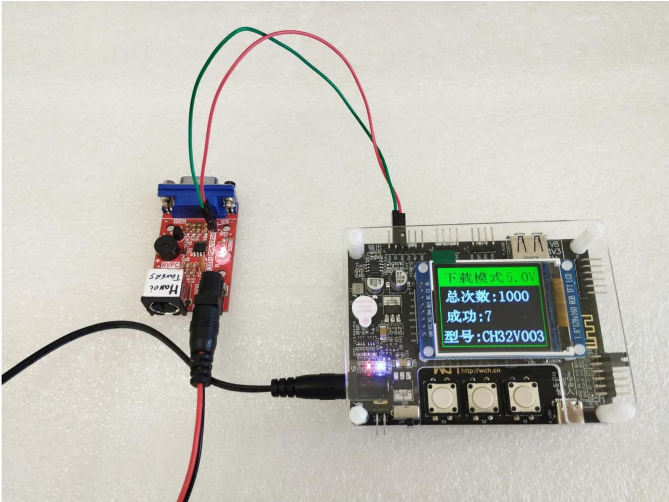
8. Programming the target via the button. Press and release button S3 (left most), then wait. This will download the code to the target board. There is info about the voltage, the programming goal (1000 times), a counter about how many times you've downloaded the binary successfully to your target/targets, and the target. Here is a video how programming goes:
